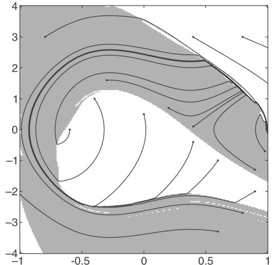
Fig. 7. Approximate optimal policy obtained for the car-on-the-hill problem. Gray and white areas indicate the maximum and minimum control values, respectively. Lines indicate some trajectories integrated using this policy. Compare to [11, Fig. 4].
