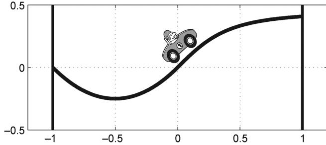
Fig. 2. Car-on-the-hill optimal control problem. The reward is identically zero inside the state space. Terminal rewards of  $-1$  and  $1 - \dot{x}/2$  are incurred upon reaching the left and right edges of the state space, respectively.
