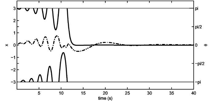
Fig. 8. Time course of the swing-up trajectory for the cart-pole dynamical system, starting from the motionless hanging-down position in the center of the track. The solid line denotes the angle of the pole and the dashed line denotes the position of the cart. Note that the horizon time scale  $\tau$  is only 1.5 s, far shorter than the total swing-up time.
