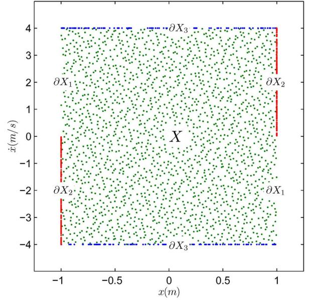
Fig. 3. Illustration of the points where the HJB residual was measured and minimized. Clamping constraints were applied to points on the “outbound”  $\partial X_2$  by minimizing  $(V(\mathbf{x}) - r(x))^2$ . For points on  $\partial X_3$ , the dynamics were modified to never point outside the state space.
