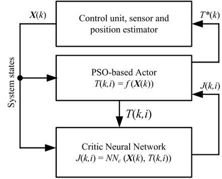
Fig. 3. General block diagram of the ADHDP dynamic sleep scheduler (sleep cycle  $k$ , PSO iteration  $i$ ).
