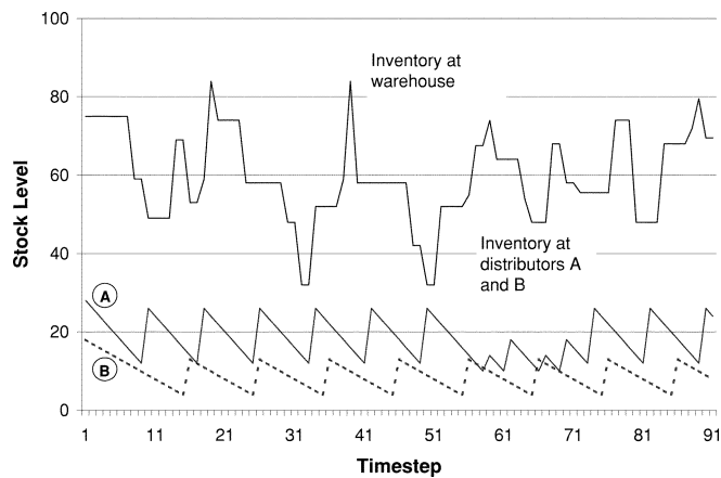
Fig. 3. Simulation output. A single stock is held at a warehouse (upper solid line), which supports two distributors, A (lower solid line), and B (lower dashed line). The inventory levels fluctuate based on the demand, the order policies, transport available, and the delivery time. As an example of the process, the warehouse shipped an order to distributor A on day seven, delivered on day nine, and shipped another to B on day nine, delivered on day 15. Between days 60 and 70, a shortage of transport kept distributor A from getting a full replenishment.
